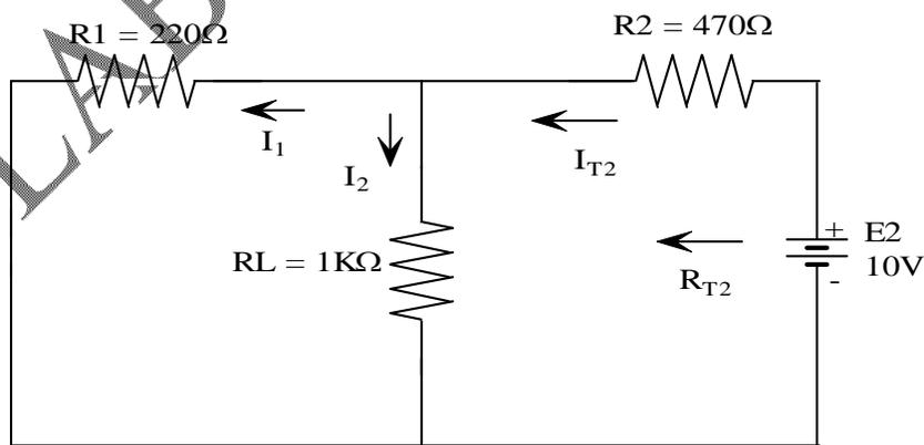
Figure.3 Considering the effect of E2 (10 V) source
