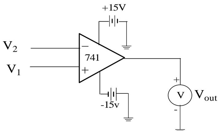
Figure.10 Practical circuit for Comparator
