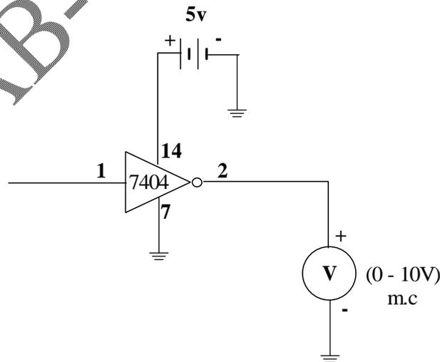
Figure.9 Practical Circuit for verification of NOT Gate
