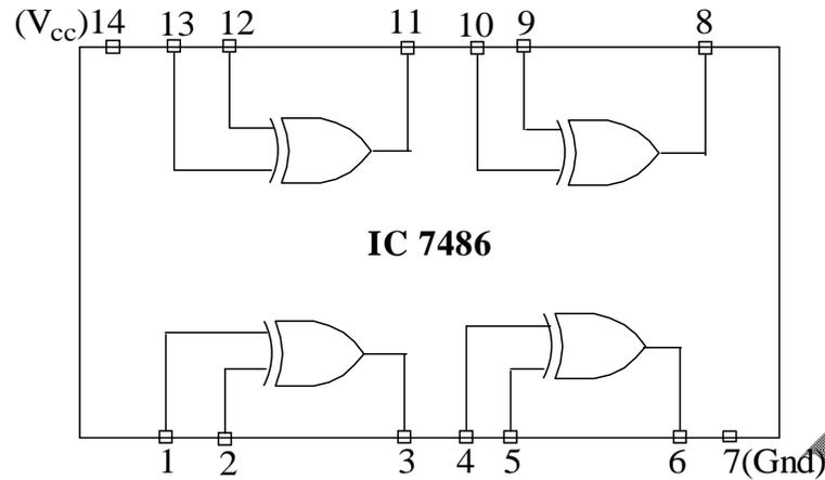
Figure.12 Pin Detail of IC 7486(XOR gate)
