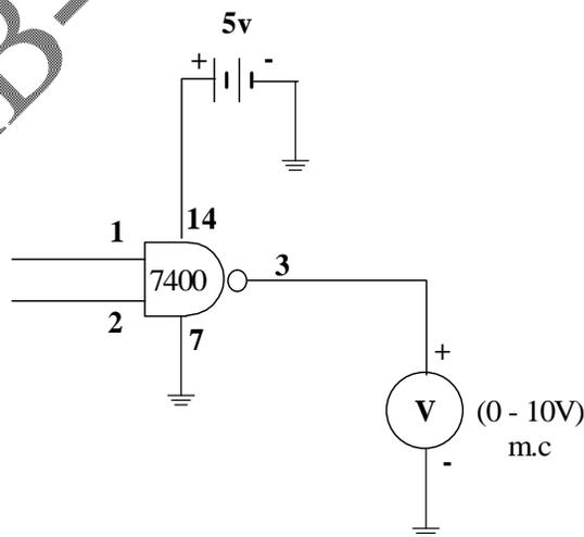
Figure.5 Practical Circuit for verification of NAND Gate
