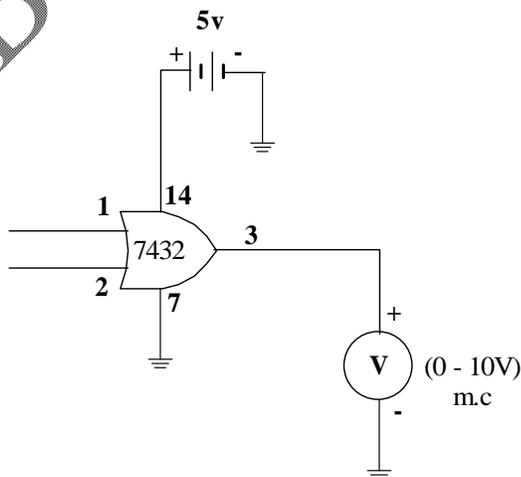
Figure.3 Practical Circuit for verification of OR Gate
