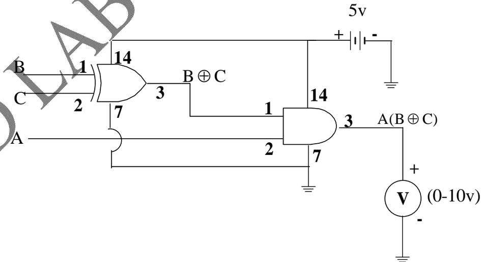
Figure.8 Implementation of Function F3 using IC 7486 and IC 7408
