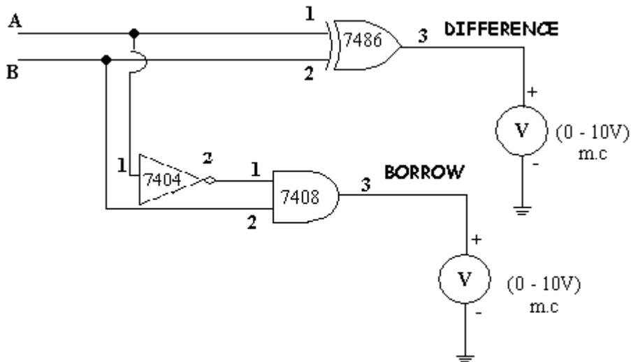
For IC's 7486, 7404 and 7408 connect pin 14 to +5v and pin 7 to Grd
