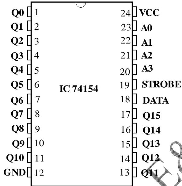
**Figure.3 Pin Diagram of Digital De multiplexer**
