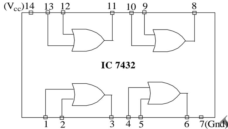
Figure.4 Pin Detail of IC 7432(OR gate)
