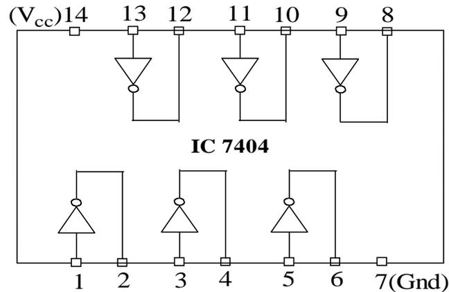
Figure.10 Pin Detail of IC 7404(NOT gate)
