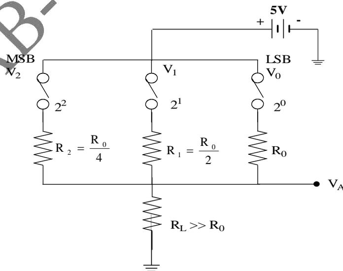
Figure.3 Resistive Divider Network
