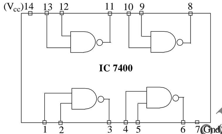
Figure.6 Pin Detail of IC 7400(NAND gate)
