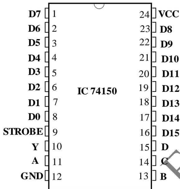
Figure.1 Pin Diagram of Digital Multiplexer
