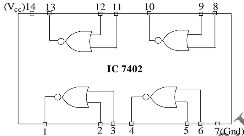
Figure.8 Pin Detail of IC 7402(NOR gate)
