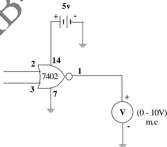
Figure.7 Practical Circuit for verification of NOR Gate
