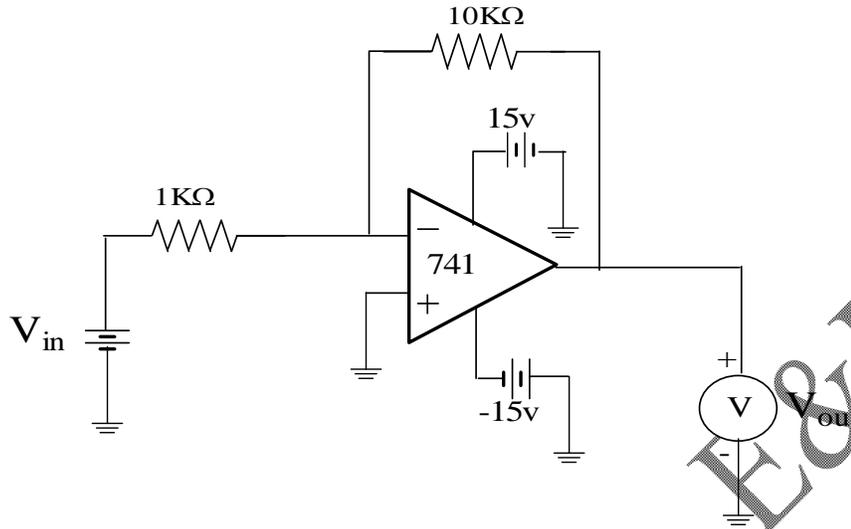
**Figure.2 Practical circuit for Inverting Amplifier**
