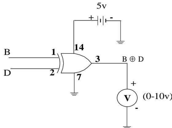
**Figure.4 Implementation of Function F1 using IC 7486**
