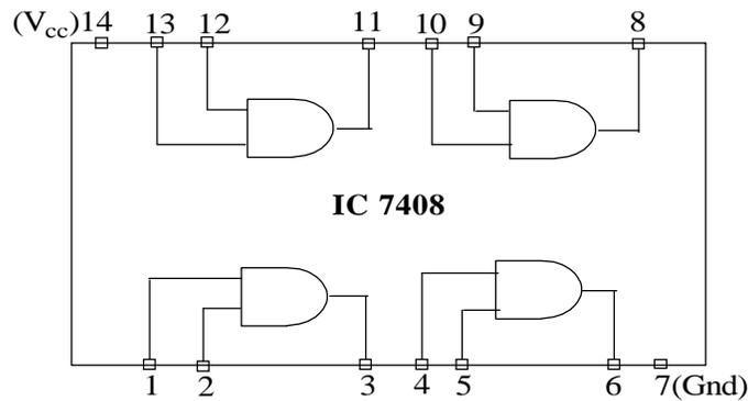
Figure.2 Pin Detail of IC 7408(AND gate)
