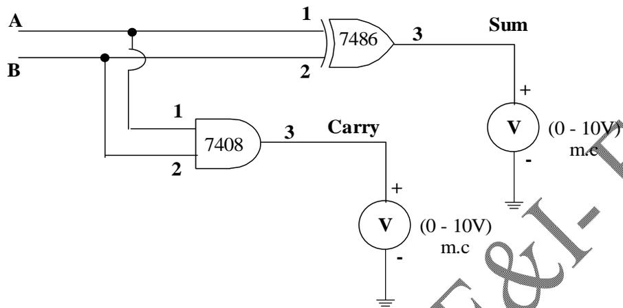
For IC's 7486 and 7408 connect pin 14 to +5v DC and pin 7 to Grd
