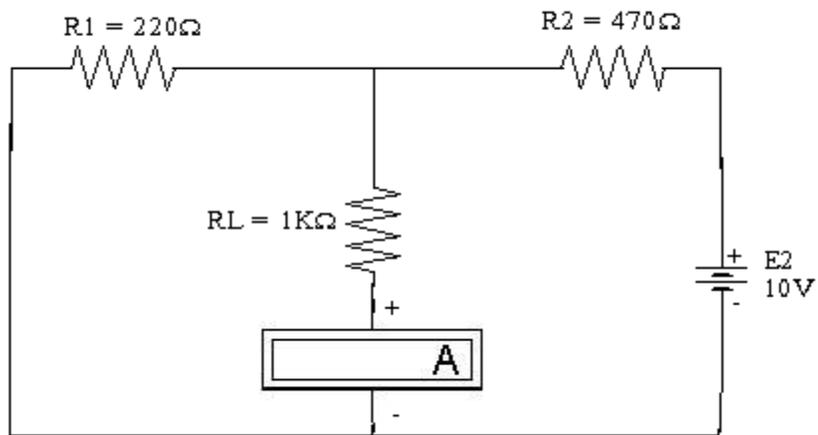
Figure.5 Connection diagram for determination of  $I_{L2}$
