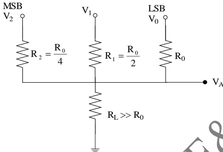
Figure.2 3-Bit Resistive Network
