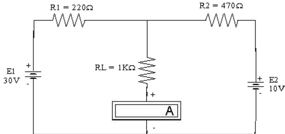
**Figure.6 Connection diagram for determination of  $I_L$**
